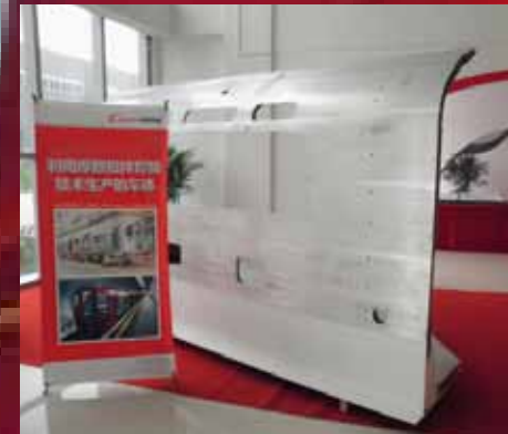
A part of a metro car body, made of several kinds of profiles.
